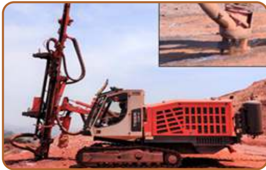
Wet drilling at Mine
