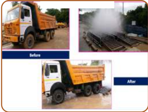
Wheel Washing system
